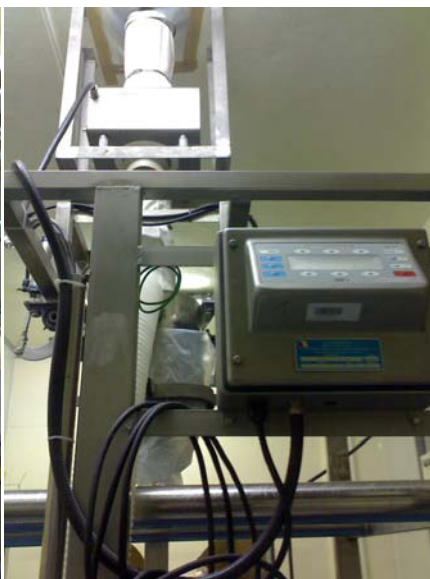
Bulk Bag Loading Station for Coffee-mate with metal detector
