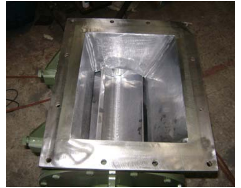
SIZE 14.0" ,carbon steel, for wood dust, pneumatic conveying system, plywood factory 100 % fit on the place of the existing unit from MOTAN
