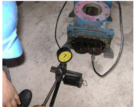
Super High pressure hydraulic hand pump "SKF", 45000 PSI ,for gear disassemble
