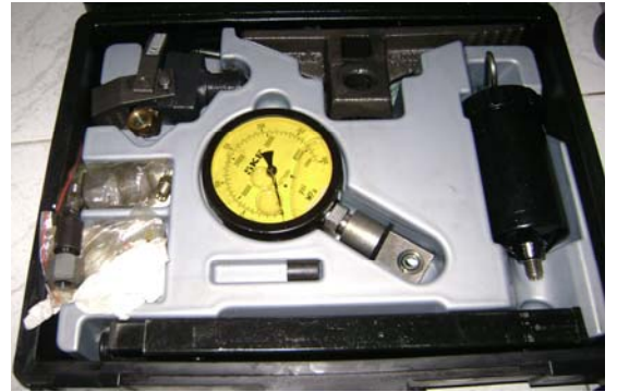
Super High pressure hydraulic hand pump "SKF", 45000 PSI ,for gear disassemble
