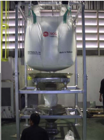
Bulk Bag Unloading Station for EVA powder
