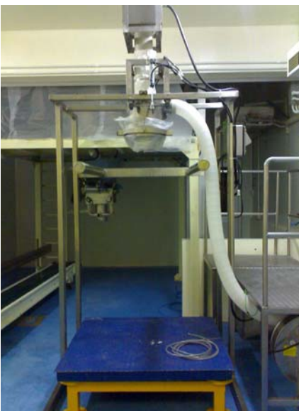
Bulk Bag Loading Station for Coffee-mate with metal detector
