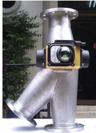
Low pressure , Corn flakes pneumatics conveying system, SUS 304, Size 100 mm
