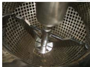
Vertical Shaft Machine for Crispy Product ( Product : Corn flake )
