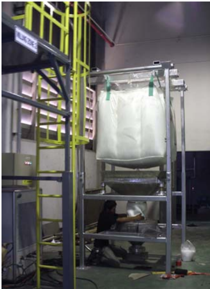
Bulk Bag Unloading Station for EVA powder
