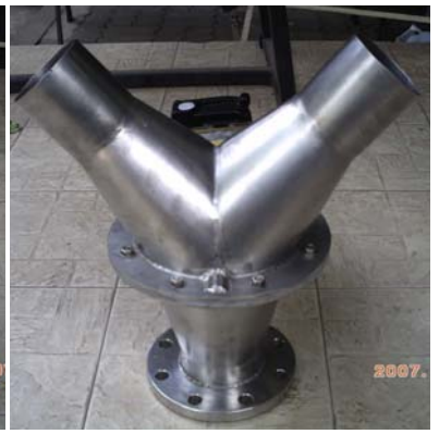
Silo Diverter Valve, For EVE, SUS 304, Size 100 mm
