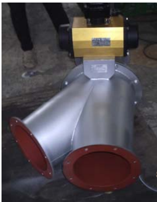
Paper Trim removal system , Carbon steel, Size 200 mm
