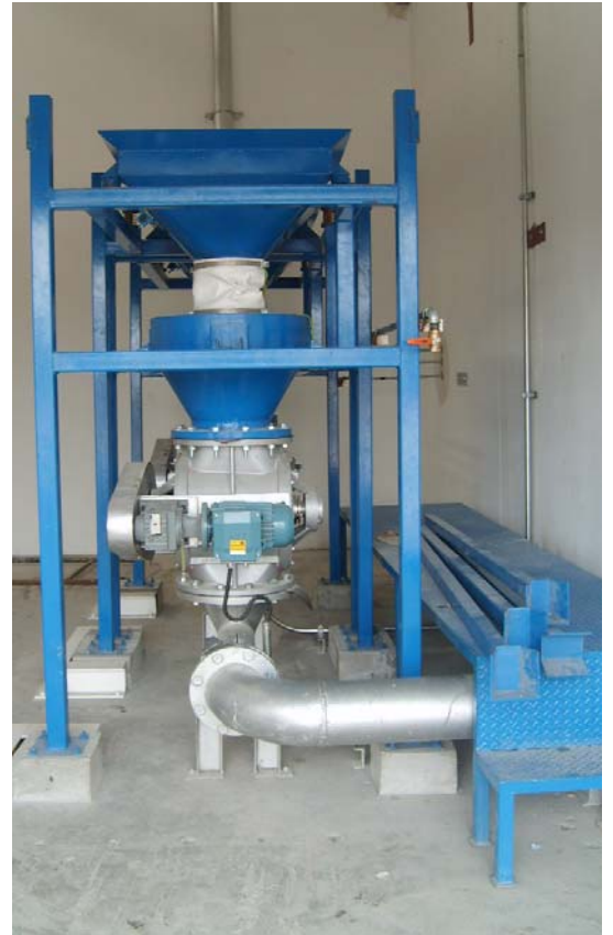
Bulk Bag Unloading Station for Bentonite clay powder
