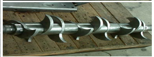
Horizontal Shaft Machine for Relatively hard Product ( Product : Rice flour lump )
