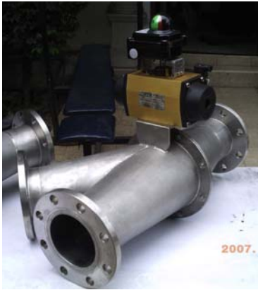
Low pressure , Corn flakes pneumatics conveying system, SUS 304, Size 100 mm
