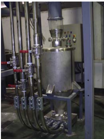
Collecting hopper & Outlet Box,SUS304
