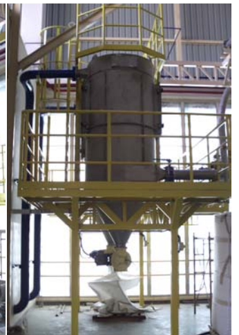
Dumping Hopper ,Ejector , Flexible hose, and Quick coupling from Extruder
